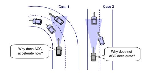
**Fig. 1** Automation surprises caused by the adaptive cruise control (ACC) system
